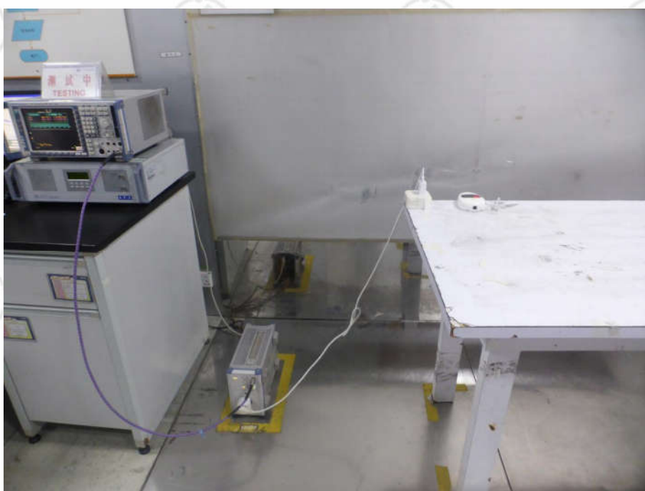
Conducted Emissions Test Setup
