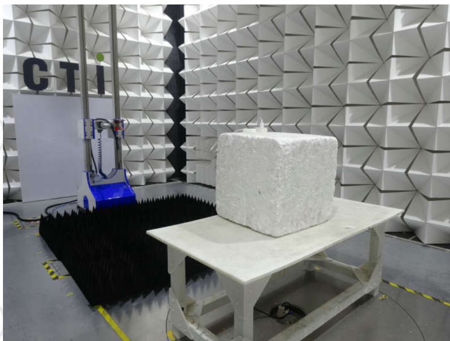
Radiated spurious emission Test Setup-2(Above 1GHz)
