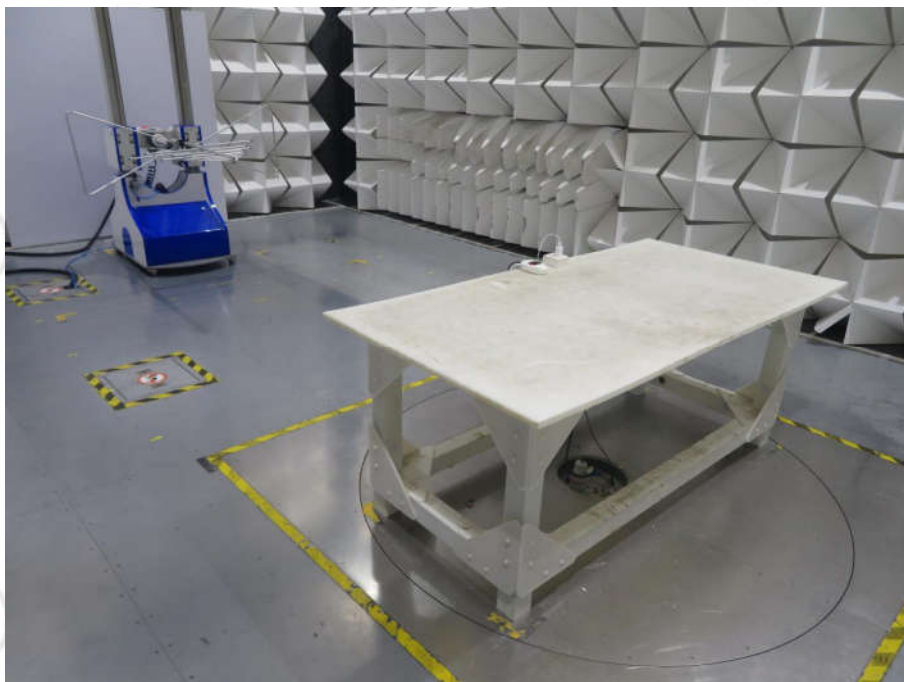
Radiated spurious emission Test Setup-1 (Below 1GHz)
