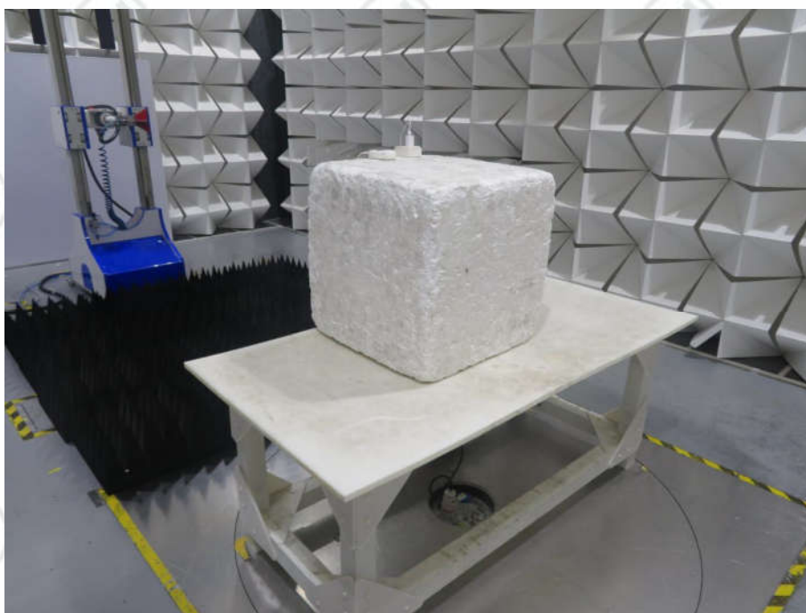
Radiated spurious emission Test Setup-2(Above 1GHz)
