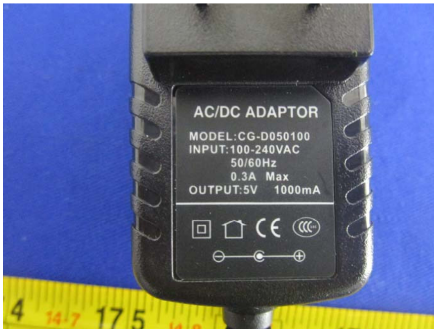
EUT- Adapter Label View
