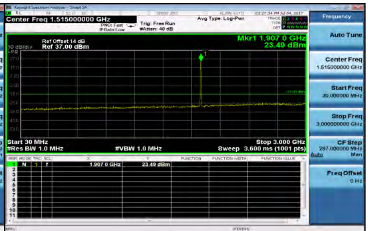
Out of Band Emission High_WCDMA_B2_LowCH9262-1852.4
