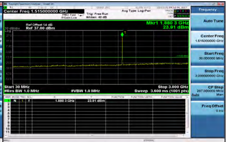
Out of Band Emission Low_WCDMA_B2_HighCH9538-1907.6
