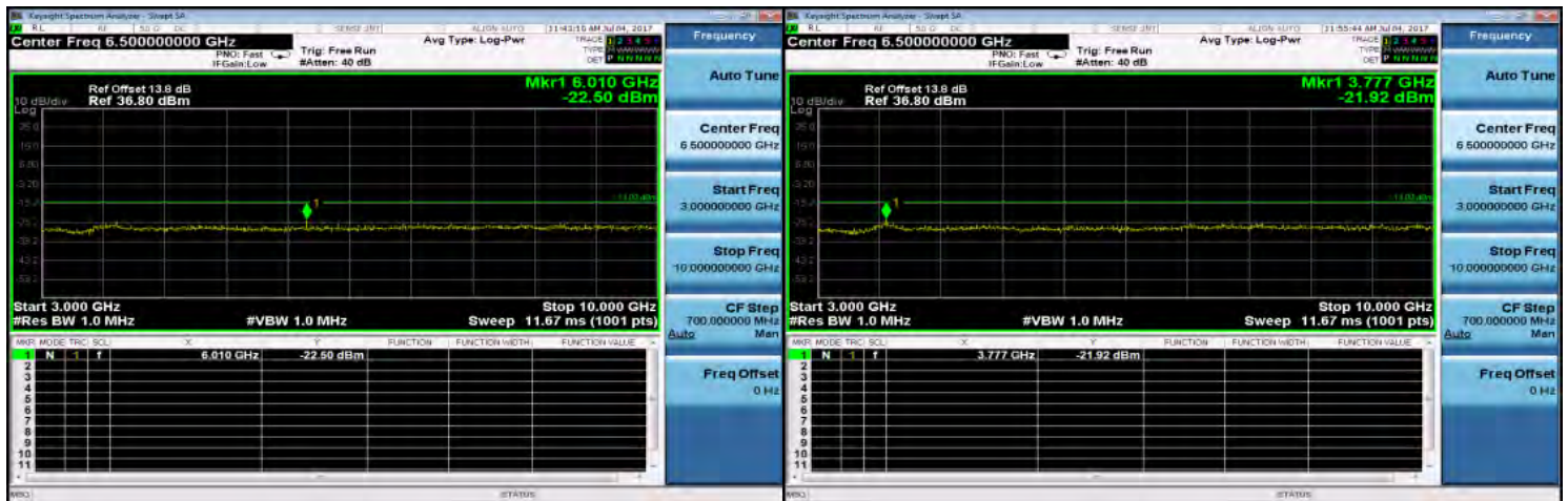
Out of Band Emission High_GPRS_850MHz_LowCH128-824.2
