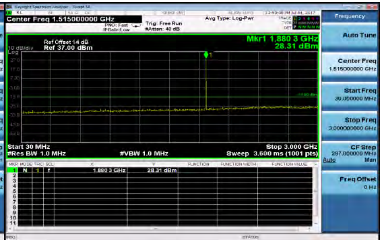
Out of Band Emission Low_EDGE_1900MHz_HighCH810-1909.8
