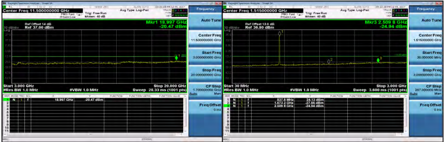
Out of Band Emission Low_WCDMA_B2_HighCH9538-1907.6
