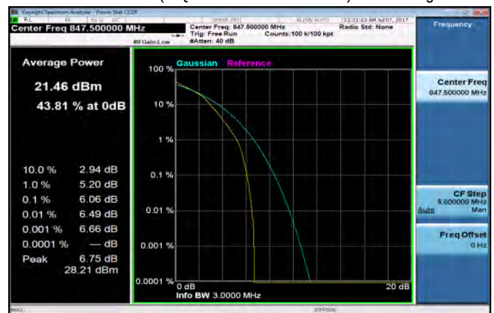
3MHz BW LTE-Band 5(16QAM Number: 15 Offset: 0) Channel High
