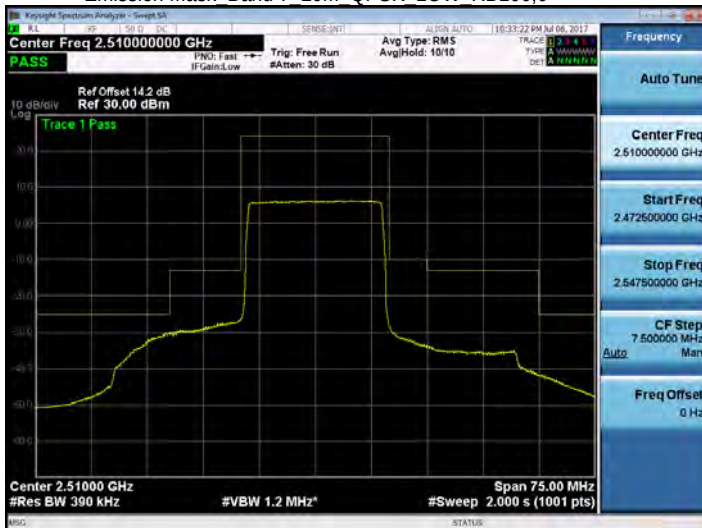
Emission Mask Band 7 20M QPSK MID RB1,0
