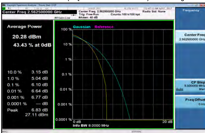
15MHz BW LTE-Band 7(16QAM Number: 75 Offset: 0) Channel High
