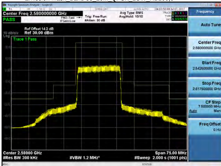
Emission Mask Band 38 20M QPSK MID RB1,0
