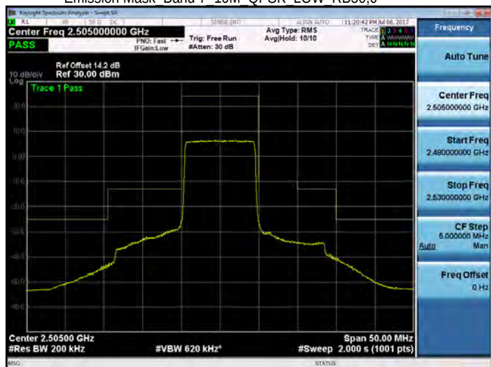
Emission Mask Band 7 10M QPSK MID RB1,0
