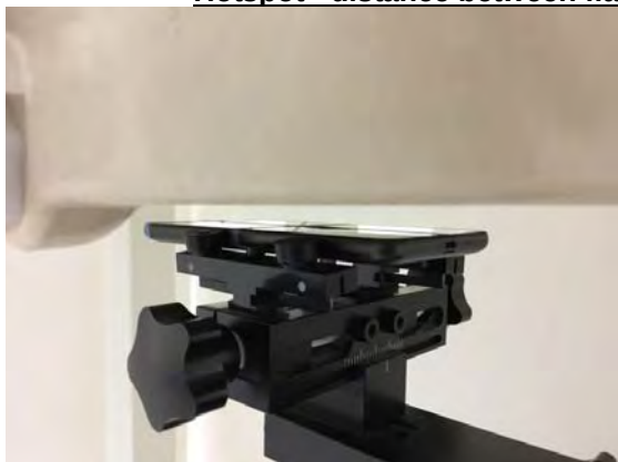
Fig.9 EUT Front side to flat phantom
