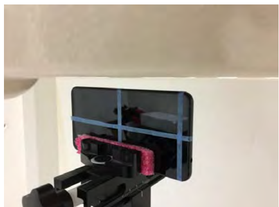
Fig.14 EUT Left side to flat phantom
