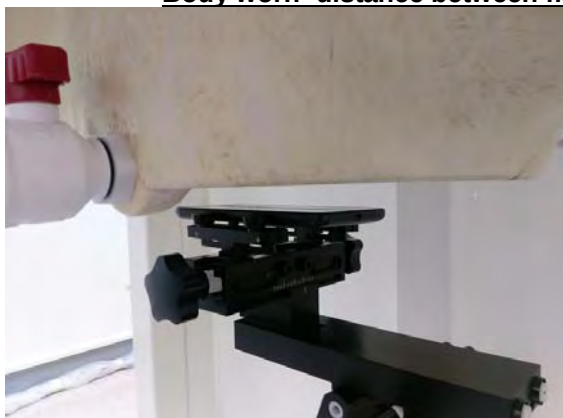
Fig.7 EUT Front side to flat phantom
