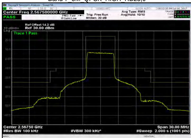
Band 7 5M QPSK HIGH RB25,0
