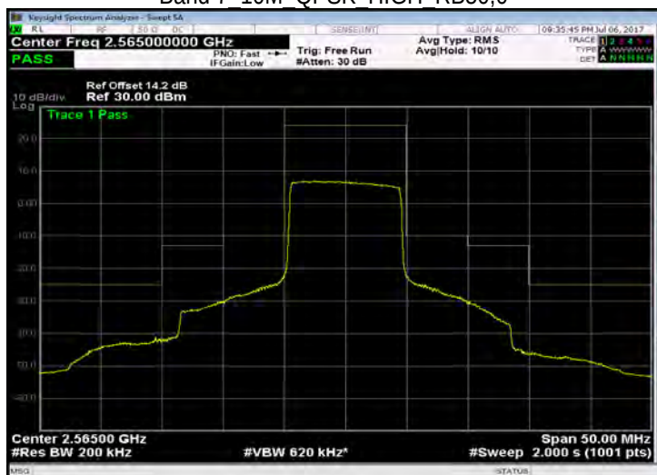
Band 7 10M QPSK HIGH RB5,0
