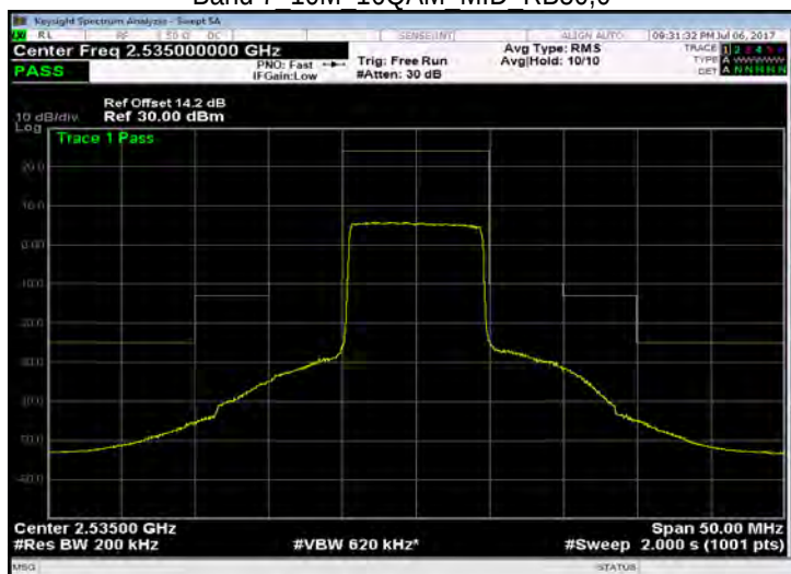
Band 7 10M 16QAM MID RB50,0
