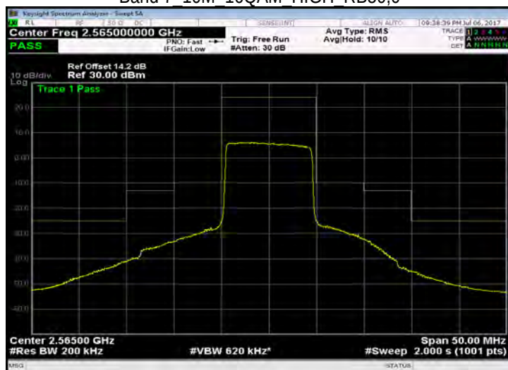
Band 7 10M 16QAM HIGH RB50,0
