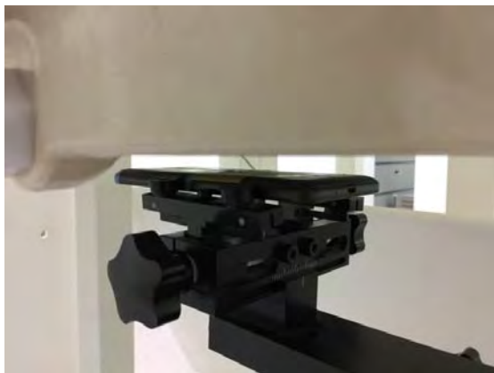
Fig.10 EUT Back side to flat phantom
