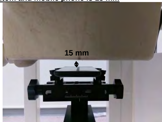
Fig.7 EUT Front side to flat phantom
