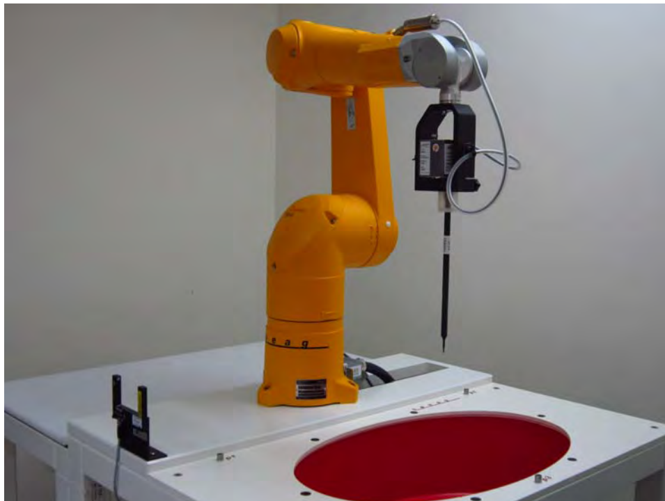
Fig.1 Photograph of the SAR measurement system
