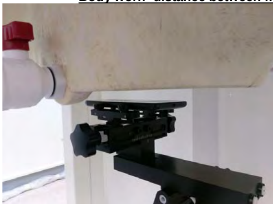
Fig.7 EUT Front side to flat phantom
