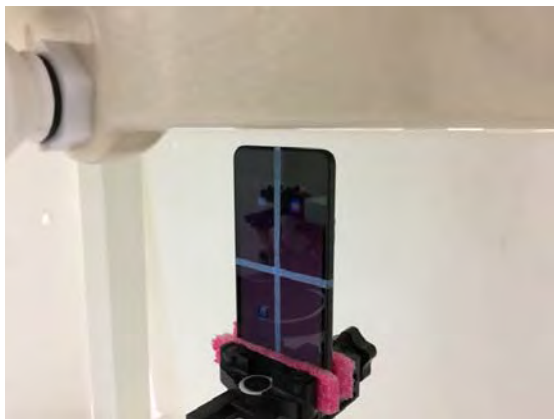
Fig.11 EUT Bottom side to flat phantom
