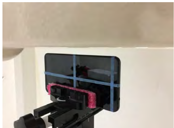
Fig.14 EUT Left side to flat phantom
