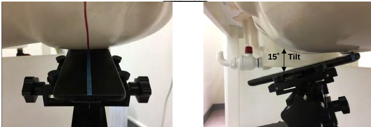
Fig.6 Left Head Section / Ear-Tilt Position(15°)
