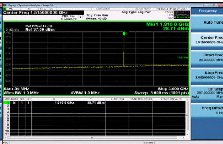
Out of Band Emission High_GSM_1900MHz_LowCH512-1850.2
