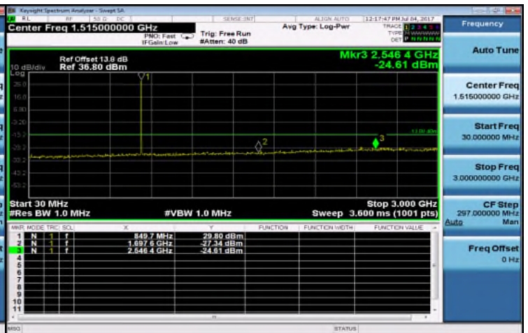
Out of Band Emission High_GSM_850MHz_LowCH128-824.2
