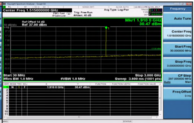
Out of Band Emission Low_GPRS_1900MHz_LowCH512-1850.2
