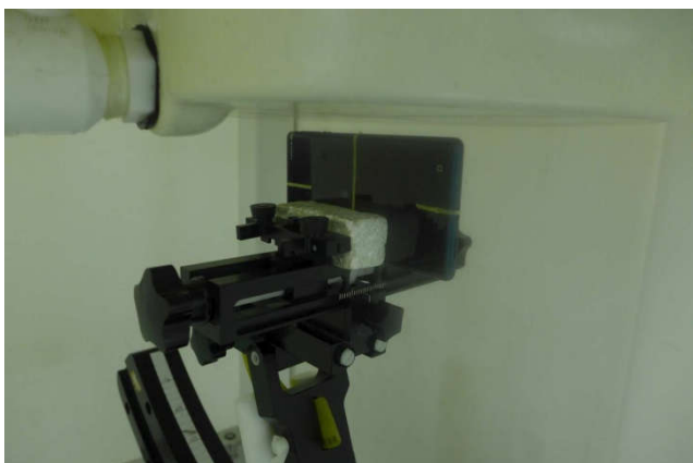
Right Side, Test Separation 10 mm
