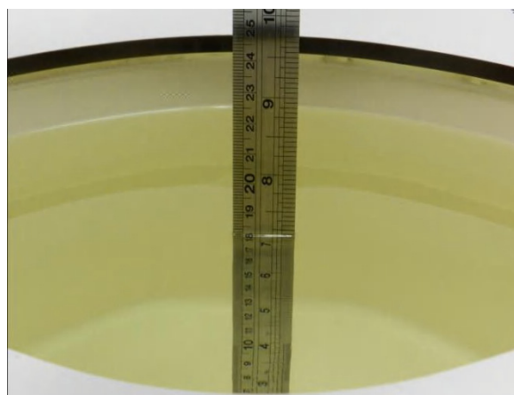
Fig 10.2 Photo of Liquid Height for Body SAR
