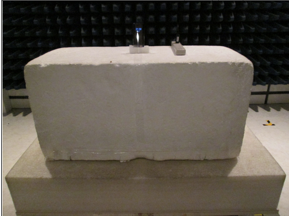
Radiated Emission Test above 1GHz (WWAN) (Z-Axis)
