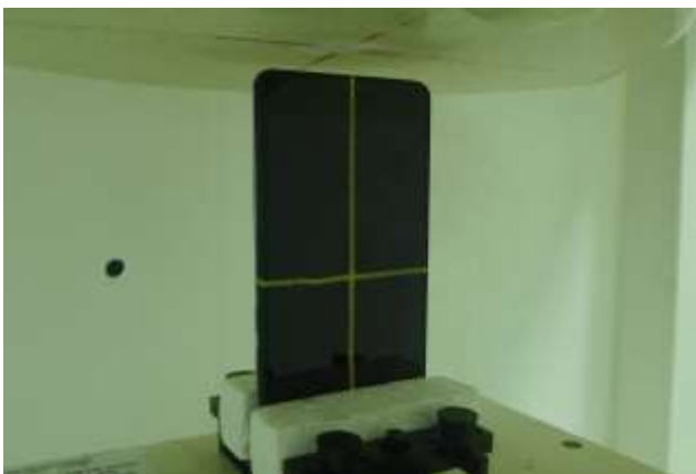
Bottom Side, Test Separation 10 mm
