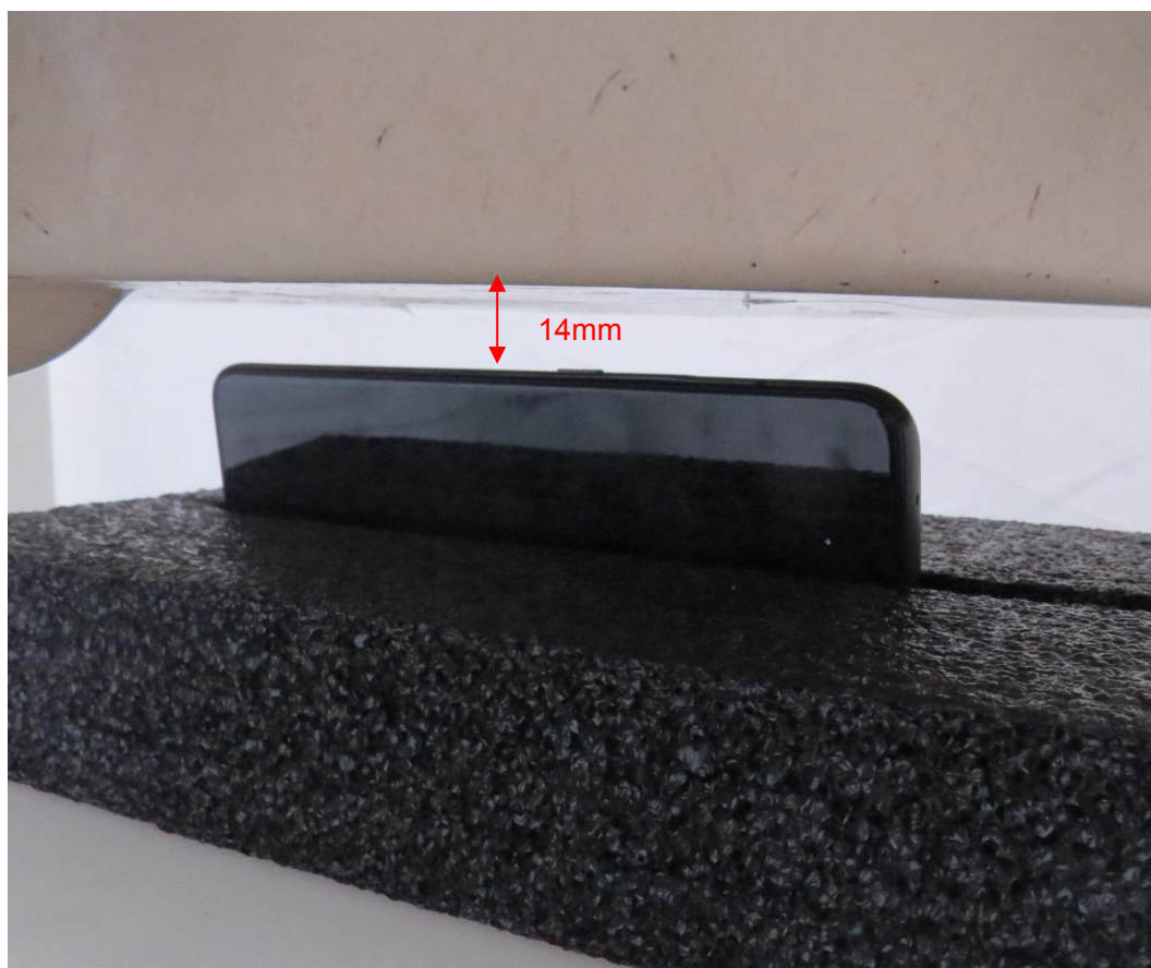
Picture 14: Left Side, the distance from handset to the bottom of the Phantom is 14mm
