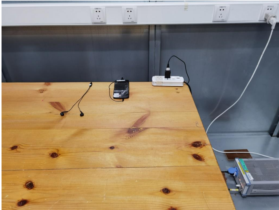
11. Conducted Emission (Part 15B, FM receiver/Camera/Video Player)
