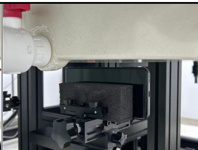
Right Side of EUT with 1.0 cm Gap
