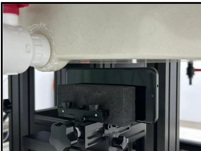
Left Side of EUT with 1.0 cm Gap
