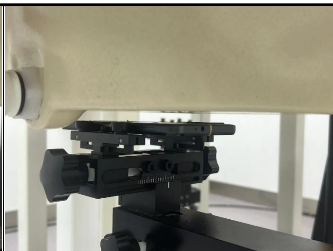
Rear Face of EUT with 1.0 cm Gap
