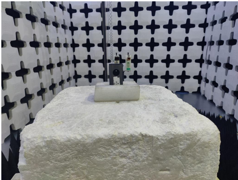
12. Radiated Emissions (Par22/24/27, 18GHz -26.5GHz)
