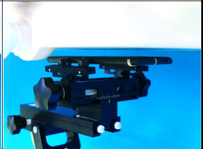
Hotspot - Rear Face of EUT at 10 mm
