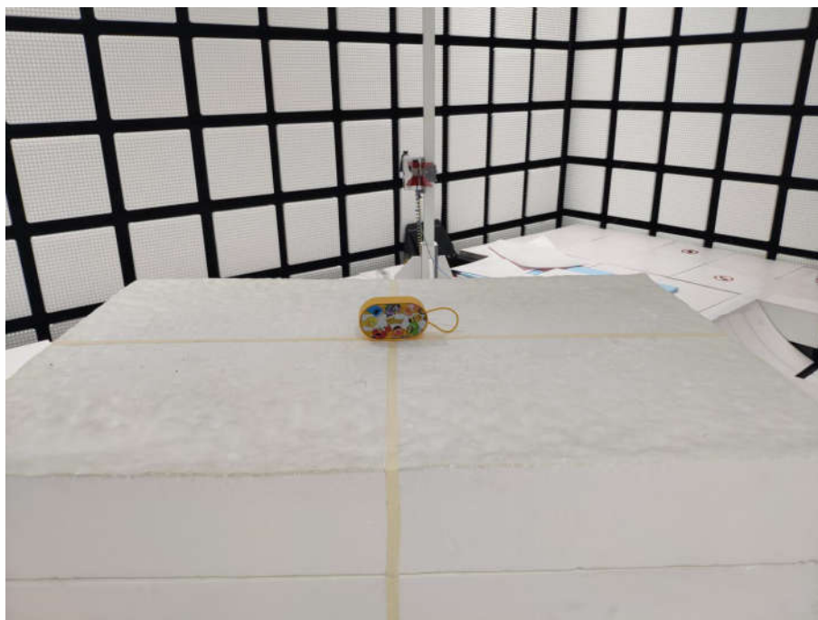
Radiated spurious emission Test Setup-3(Above 1GHz)
