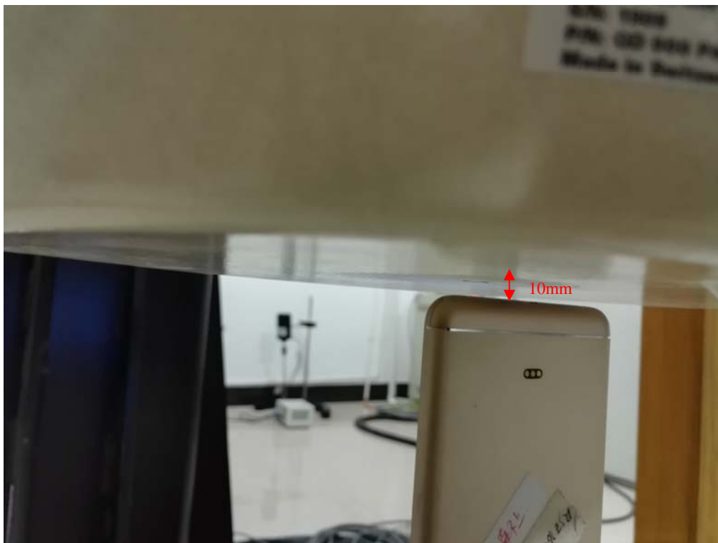
Body-worn Bottom Setup Photo (10mm)
