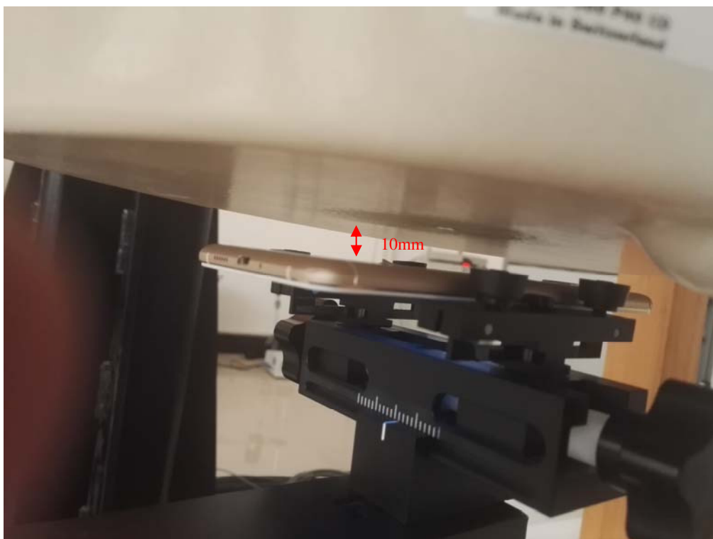
Body-worn Back Setup Photo (10mm)
