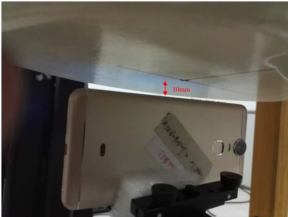
Body-worn Right Setup Photo (10mm)
