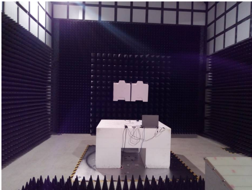
Radiated Emissions – Rear View (Above 1 GHz)
