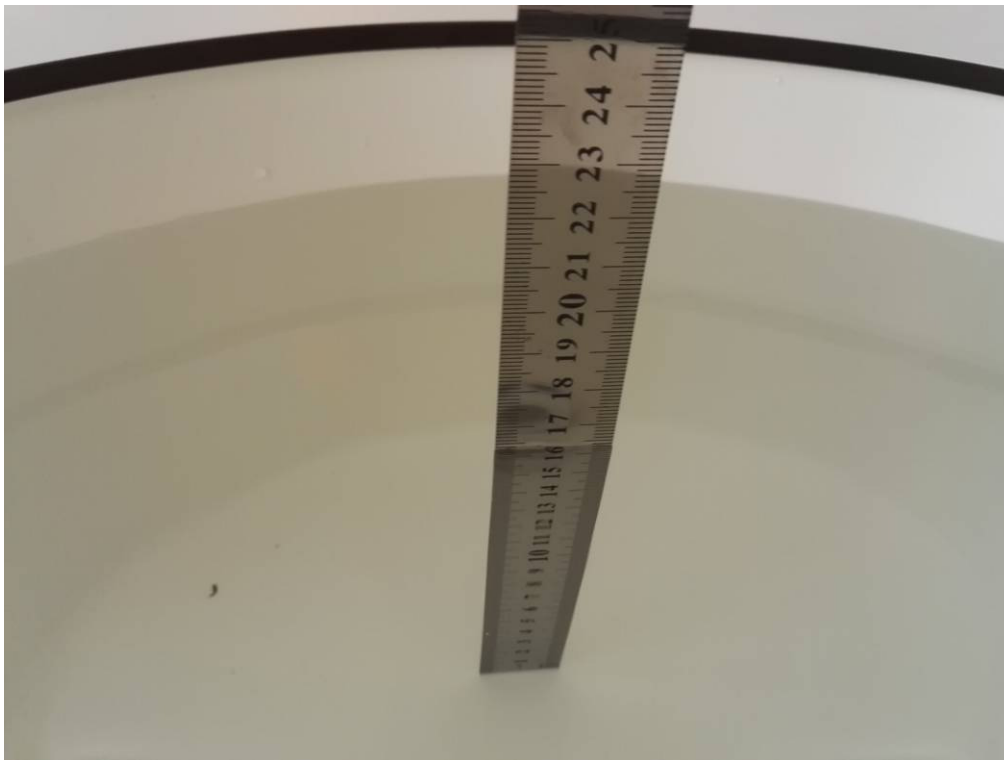
Liquid depth \geq 15\text{cm}
