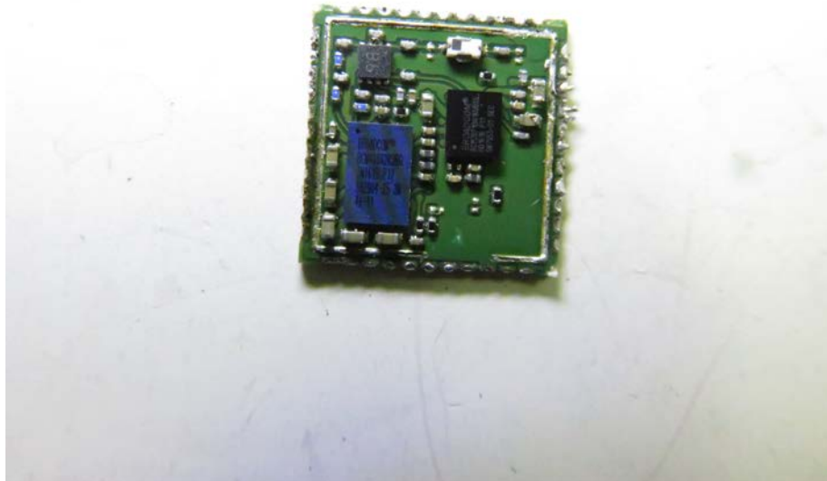
Front View of the Module (BT & WIFI)
