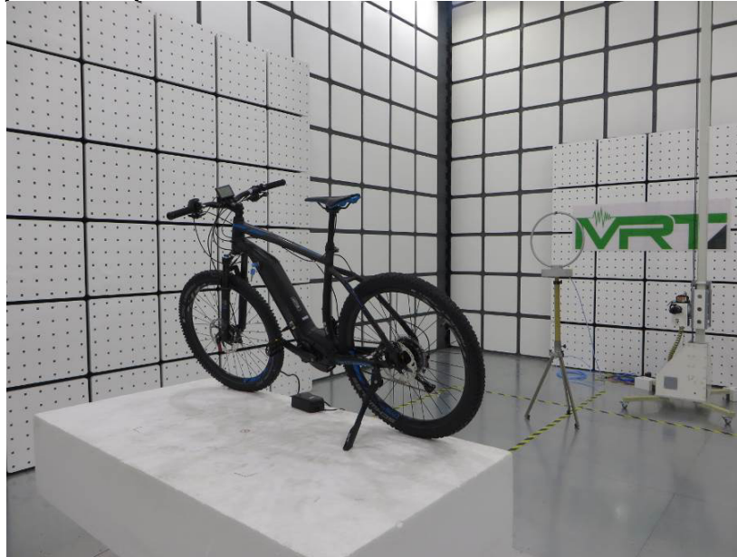
Photograph 1: Set-up for Radiated Test below 30MHz
