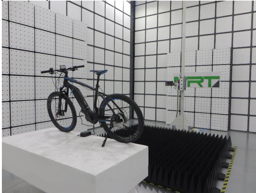
Photograph 3: Set-up for Radiated Test above 1GHz
