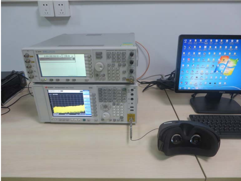
Description: Conducted Test Setup
