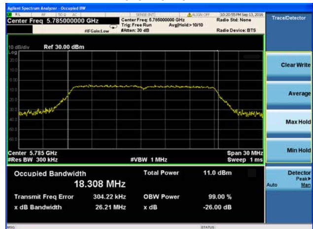
(802.11n20) -26dB&amp;99% Bandwidth plot on channel 157
