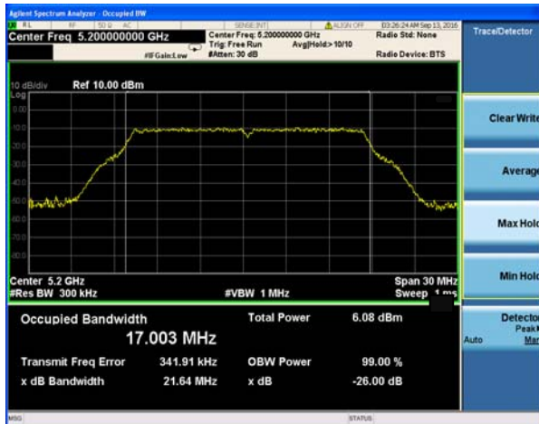
(802.11a) -26dB&amp;99% Bandwidth plot on channel 40
