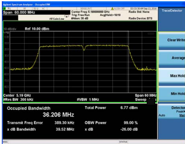
(802.11n40) -26dB&99% Bandwidth plot on channel 46
