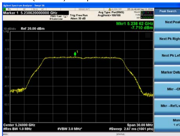
(802.11a) PSD plot on channel 48
