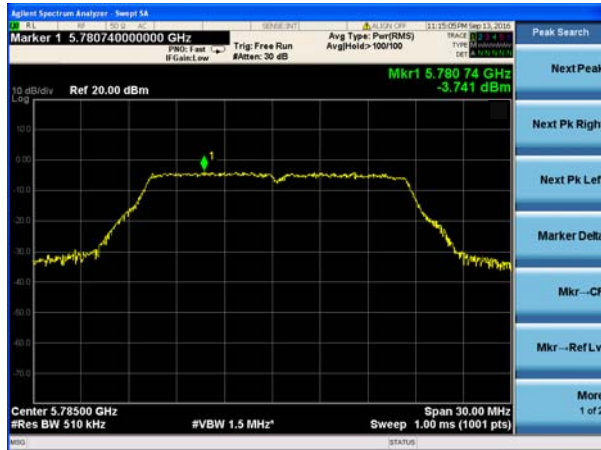
(802.11a) PSD plot on channel 157
