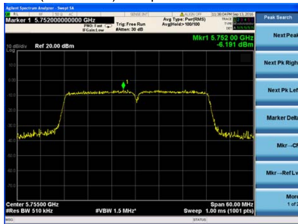
(802.11ac40) PSD plot on channel 151
