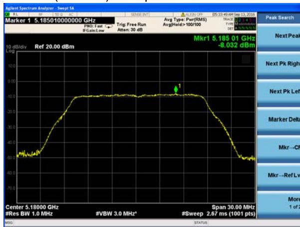
(802.11a) PSD plot on channel 36
