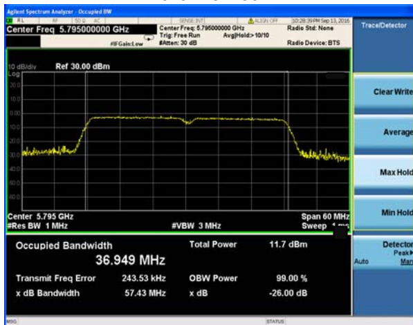
(802.11n40) -26dB&99% Bandwidth plot on channel 159
