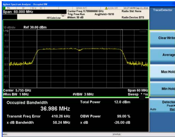
(802.11n40) -26dB&99% Bandwidth plot on channel 159
