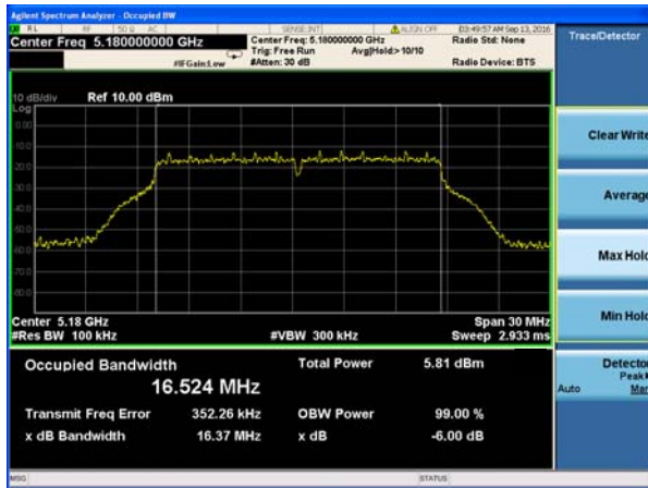
(802.11a) -6dB Bandwidth plot on channel 36
