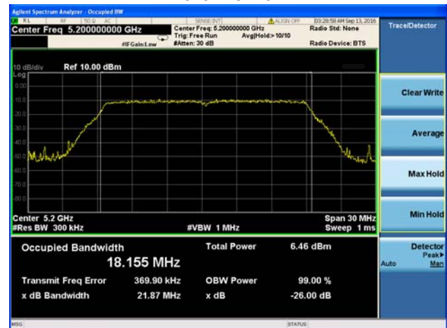
(802.11ac20) -26dB&99% Bandwidth plot on channel 40
