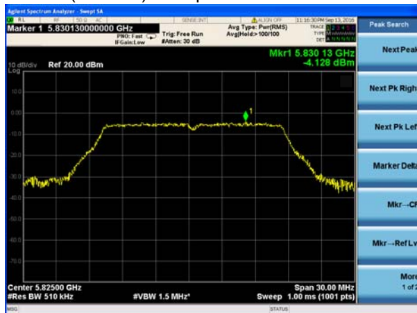
(802.11a) PSD plot on channel 165
