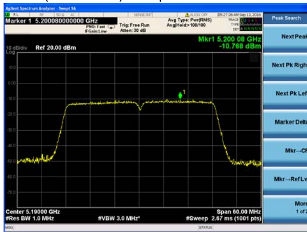
(802.11ac40) PSD plot on channel 38
