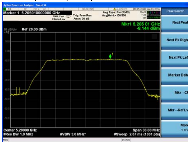
(802.11a) PSD plot on channel 40
