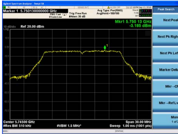
(802.11a) PSD plot on channel 149
