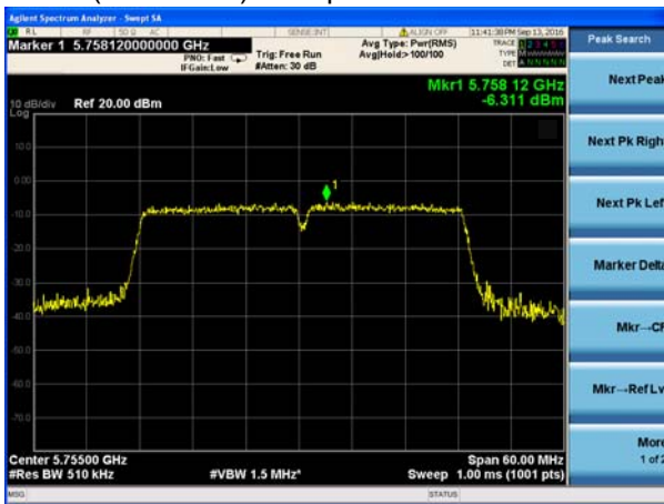
(802.11n40) PSD plot on channel 151
