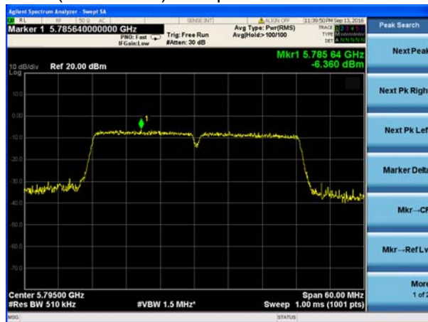
(802.11ac40) PSD plot on channel 159
