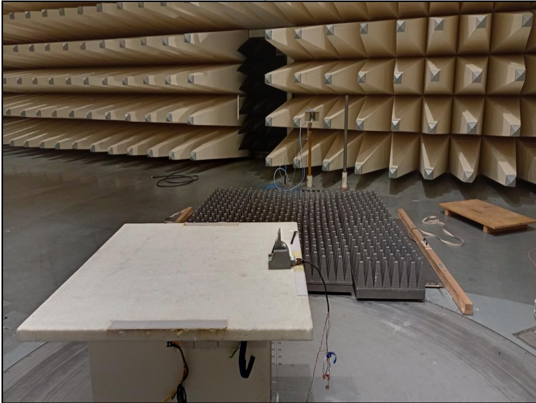
Photo 3: test setup radiated emission
