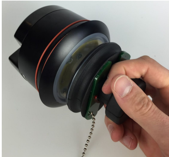
Figure 21 - Removing Faceplate from Unit
