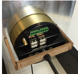
Figure 9 – Securing Subassembly Against Mounting Plate Bracket
