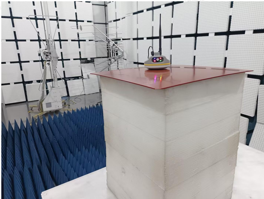
Radiated Emissions Measurement (Below 1GHz)
