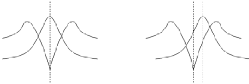
a. Peak/Null Coincident, Depth Credible b. Peak/Null Not Coincident, Depth Not Credible
