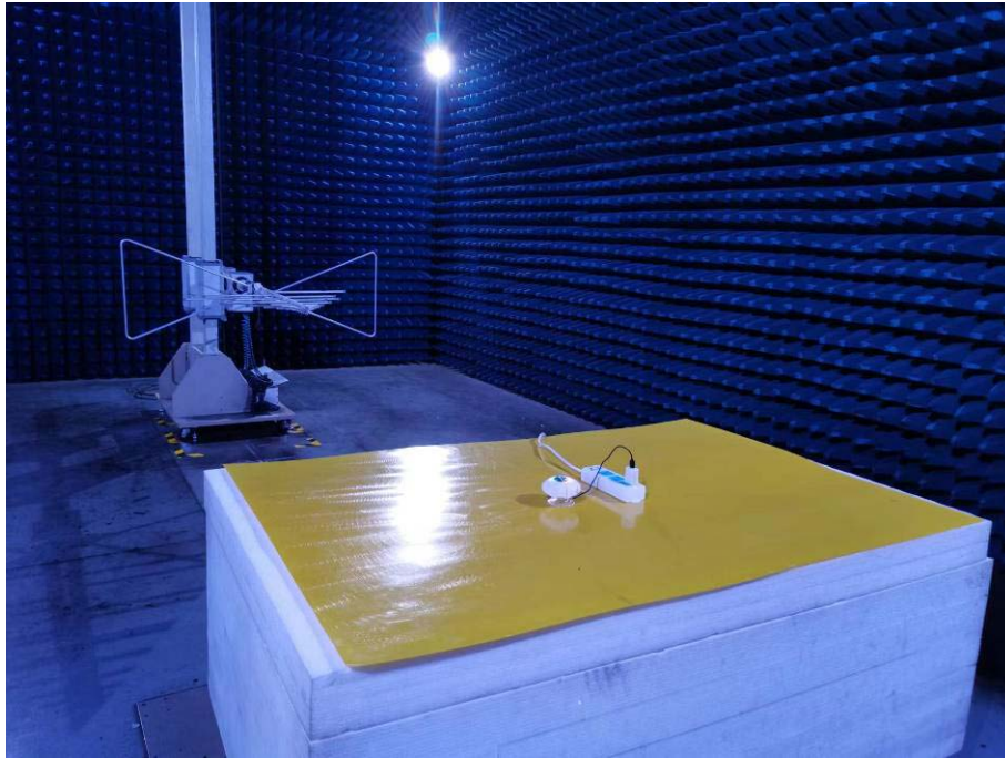
Photo of Radiated Emission Measurement Below 1GHz
