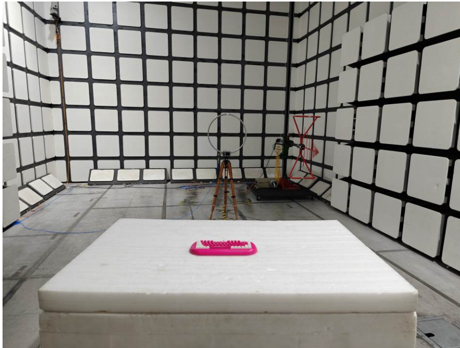
Radiated Emissions View (Below 30MHz)
