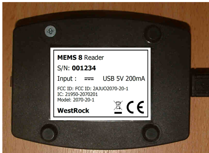
Label location (Rear side of equipment)
