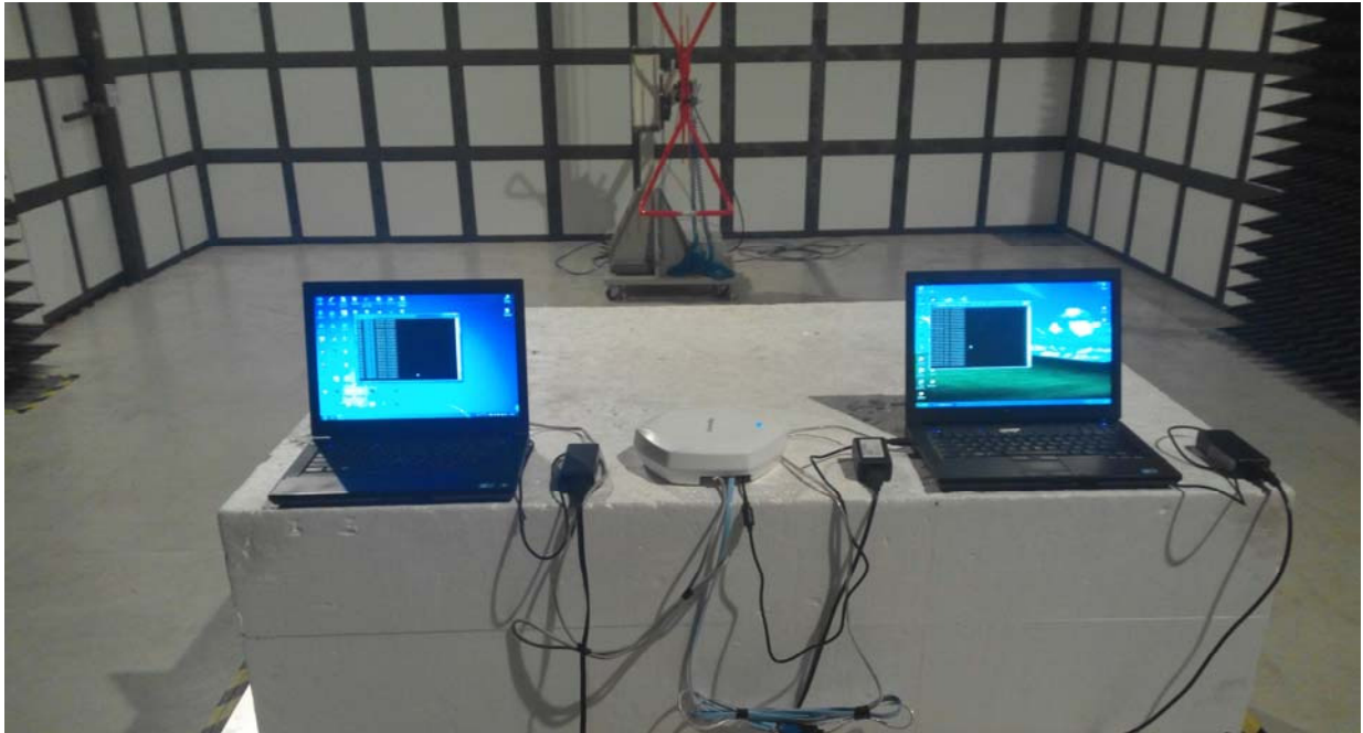
Radiated Emissions- Front View (Below 1G)
