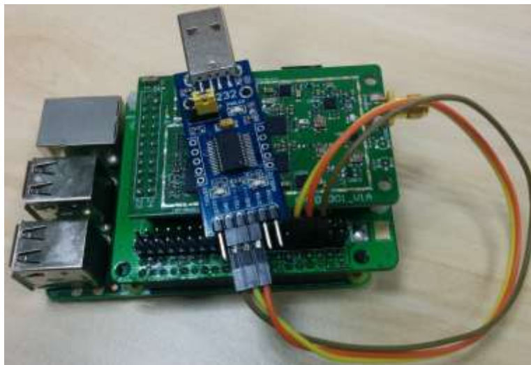
Figure 7 RPi and FT232 real product connections
