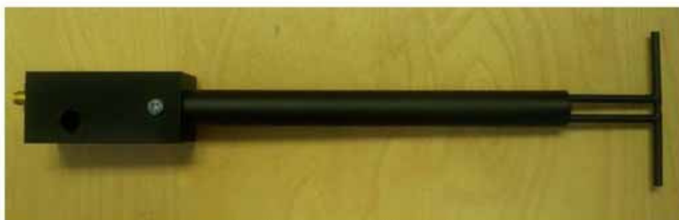
Figure 1 – MVG COMOSAR Validation Dipole
