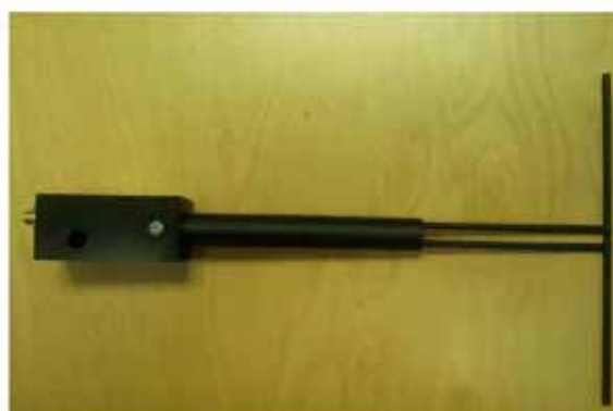
Figure 1 – MVG COMOSAR Validation Dipole
