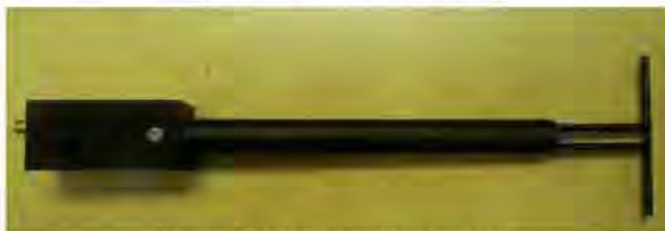
Figure 1 – MVG COMOSAR Validation Dipole
