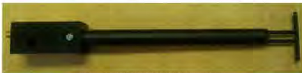
Figure 1 – MVG COMOSAR Validation Dipole
