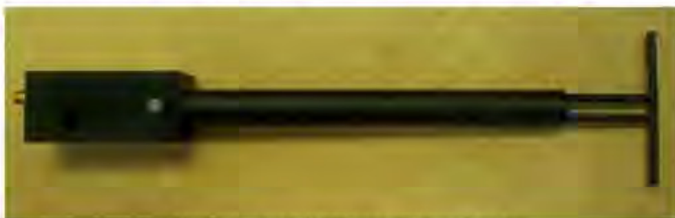
Figure 1 – MVG COMOSAR Validation Dipole
