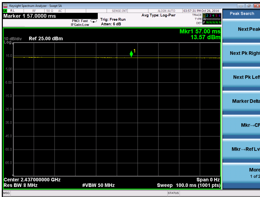
Test plot of Duty Cycle for 802.11b
