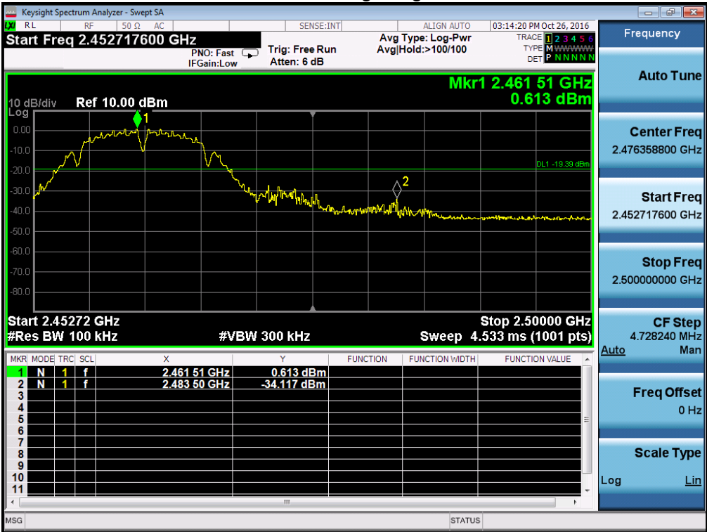
802.11b: Band Edge, high channel
