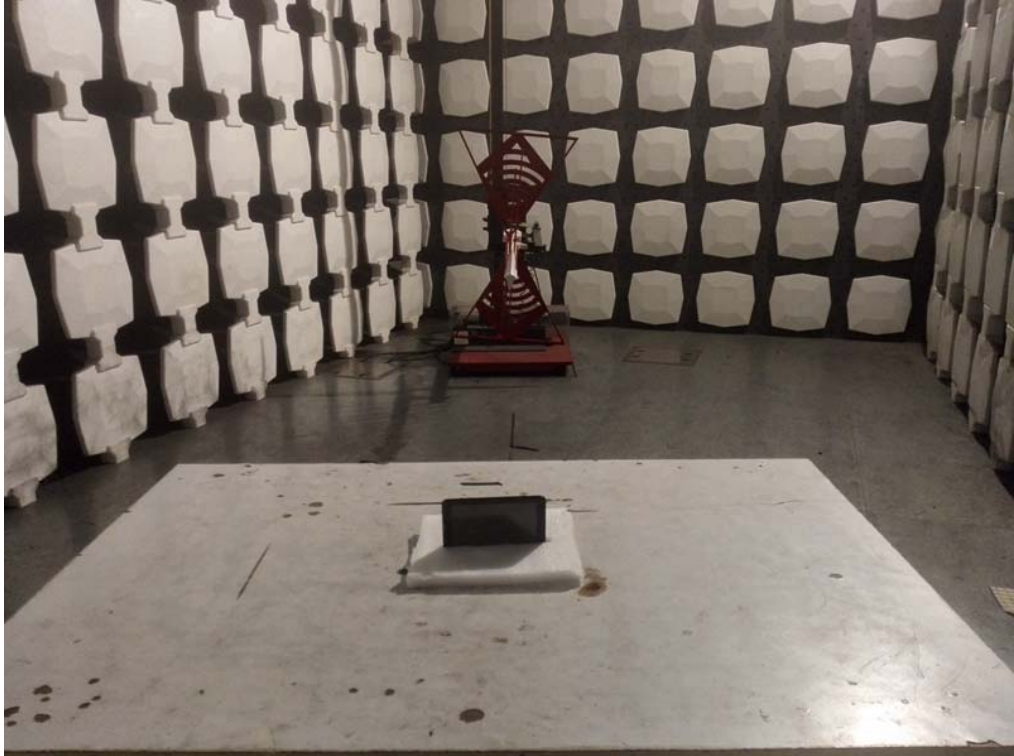
Radiated Emission Test
