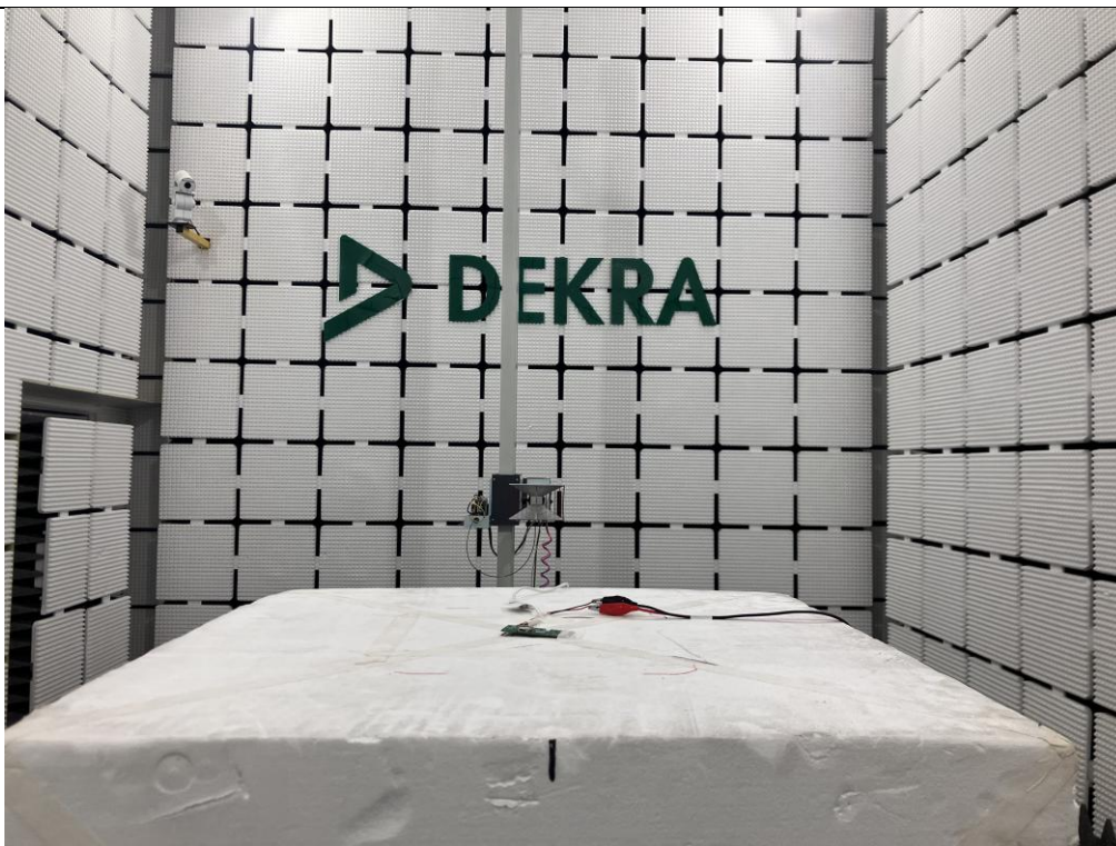
Test Location B: Radiated emission 1-18GHz
