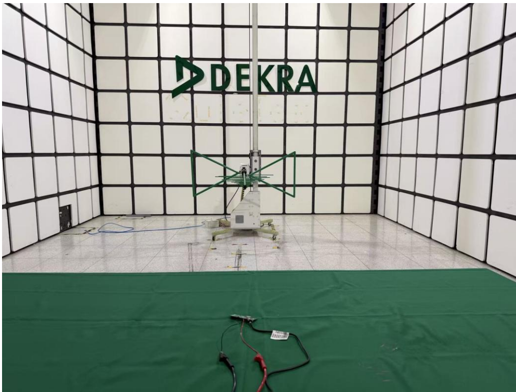
Test Location B: Radiated emission 1-18GHz
