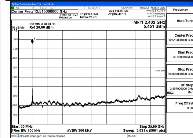
Mode:802.11ax HE40 Frequency:2422MHz Ant:Chain0
