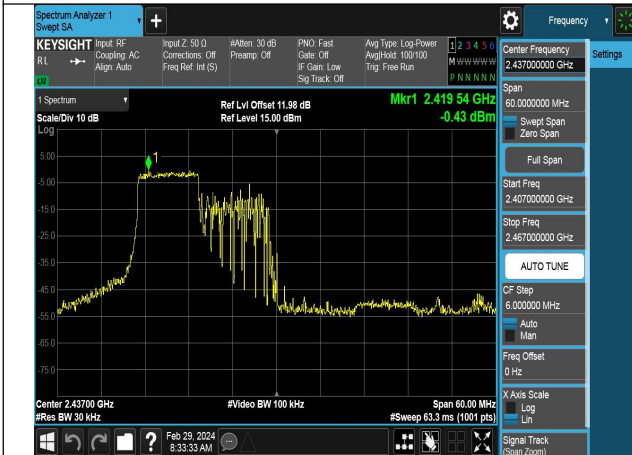
Mode:802.11ax HE40 Tone:106T Frequency:2437MHz Ant:Chain1
