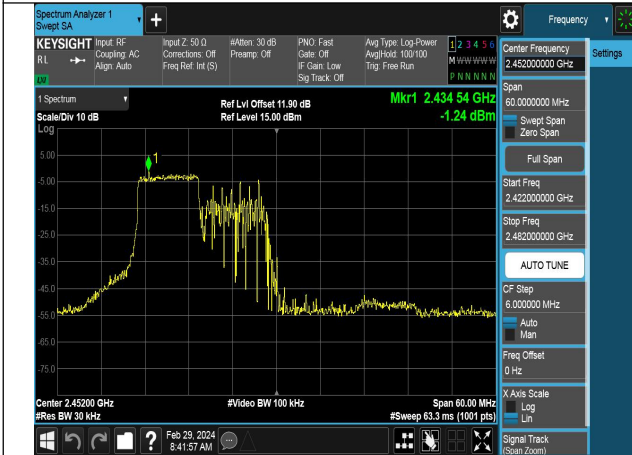
Mode:802.11ax HE40 Tone:106T Frequency:2452MHz Ant:Chain0
