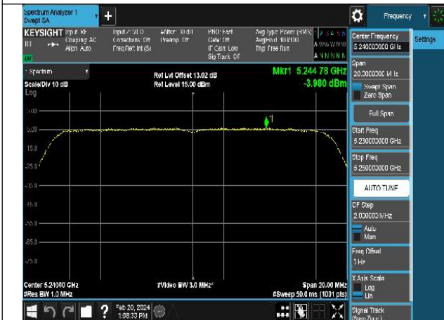
Mode:802.11ac VHT20 Frequency:5240MHz Ant:Chain0
