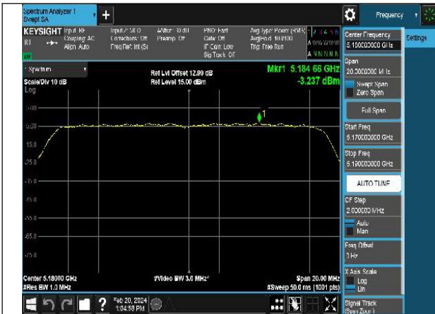
Mode:802.11ac VHT20 Frequency:5180MHz Ant:Chain0
