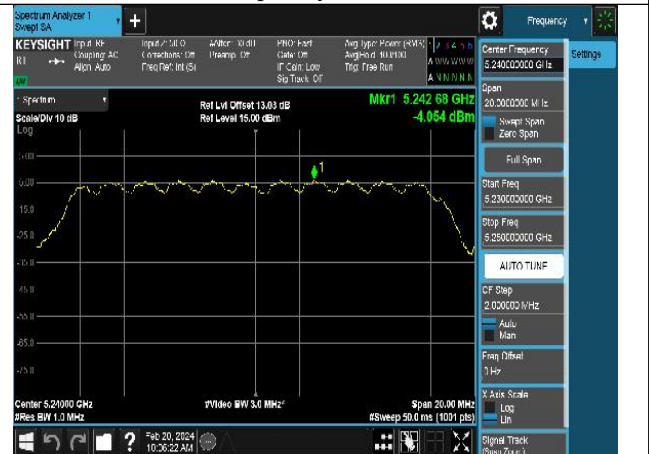
Mode:802.11a Frequency:5240MHz Ant:Chain1
