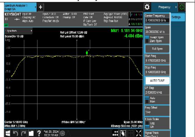
Mode:802.11a Frequency:5180MHz Ant:Chain1
