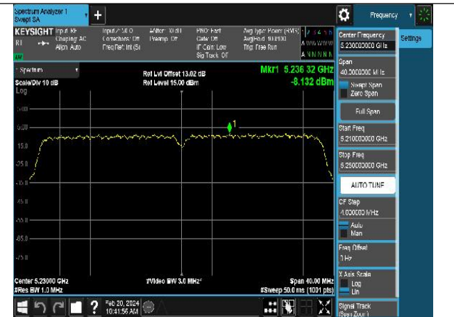
Mode:802.11n HT40 Frequency:5230MHz Ant:Chain0
