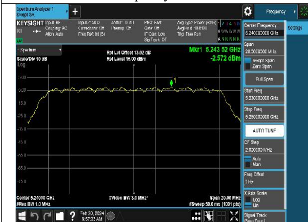
Mode:802.11a Frequency:5240MHz Ant:Chain0
