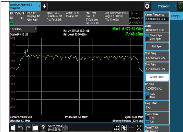
Mode:802.11n HT40 Frequency:5190MHz Ant:Chain0
