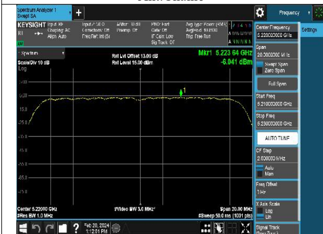
Mode:802.11ac VHT20 Frequency:5220MHz Ant:Chain1
