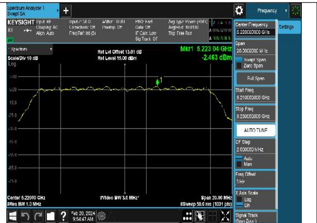
Mode:802.11a Frequency:5220MHz Ant:Chain0
