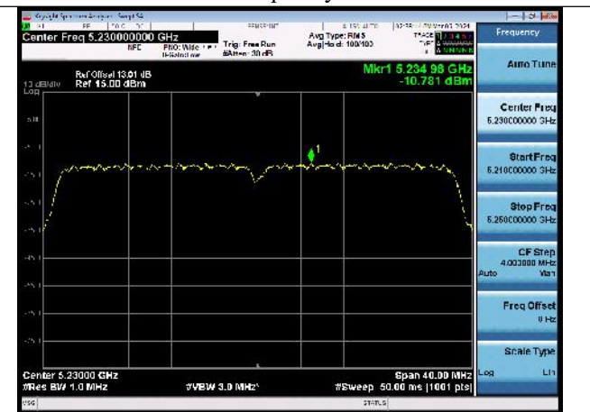
Mode:802.11n HT40 Frequency:5230MHz Ant:Chain1
