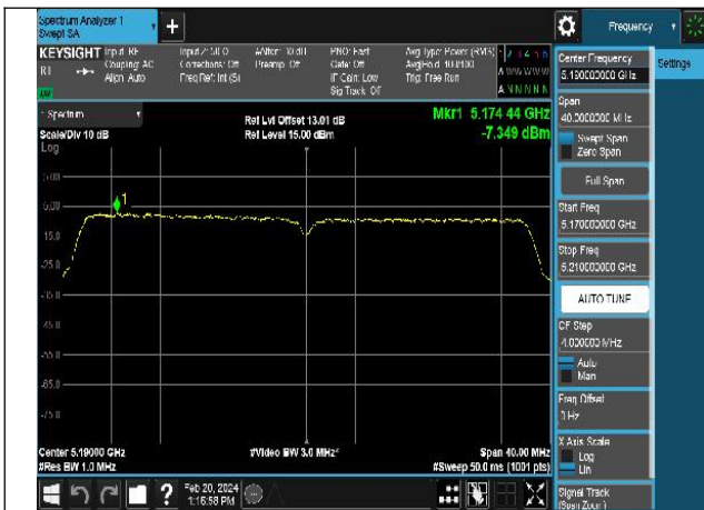
Mode:802.11ac VHT40 Frequency:5190MHz Ant:Chain0
