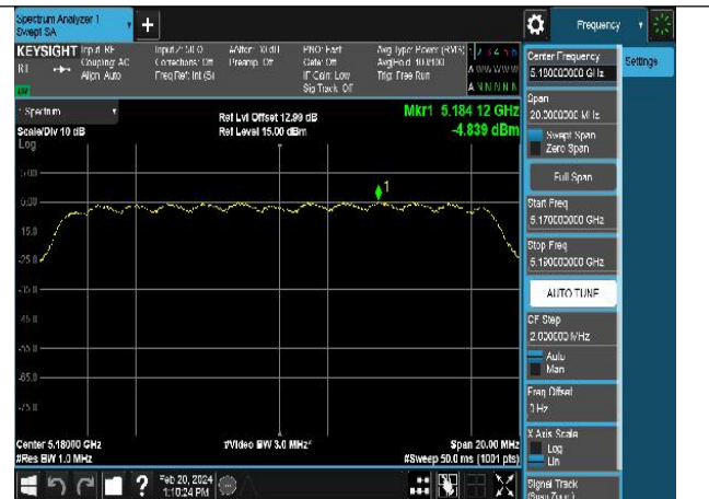
Mode:802.11ac VHT20 Frequency:5180MHz Ant:Chain1
