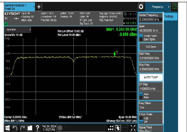
Mode:802.11ac VHT40 Frequency:5230MHz Ant:Chain0
