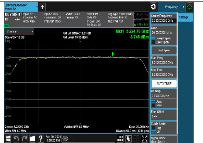
Mode:802.11ac VHT20 Frequency:5220MHz Ant:Chain0
