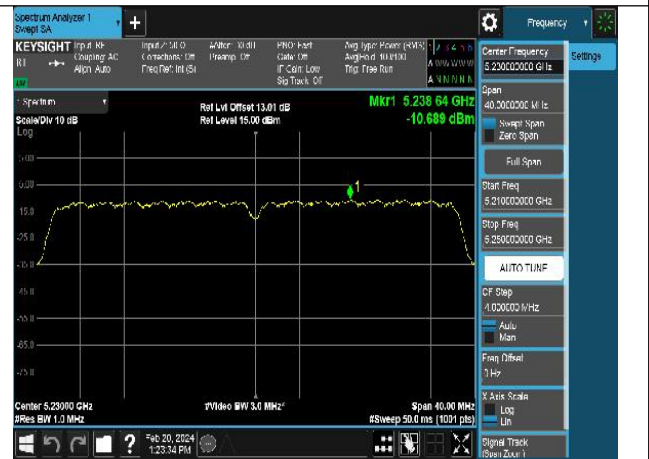
Mode:802.11ac VHT40 Frequency:5230MHz Ant:Chain1
