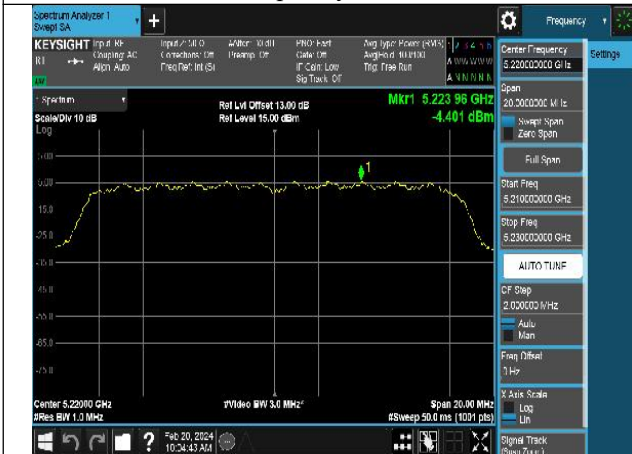
Mode:802.11a Frequency:5220MHz Ant:Chain1
