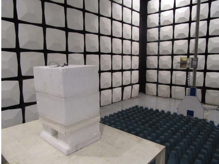
Radiated Emission View (Above 1GHz)
