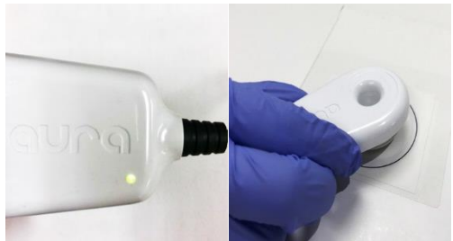
Figure 12: Positioning the AURA™ Antenna at the sticker on the AURA™ Sensor Tray box to run in-package check.
