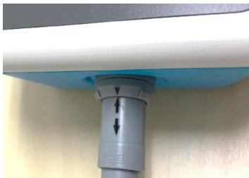
Figure 10: Align the arrow markings on the antenna cable and the AURA™ Monitor.
