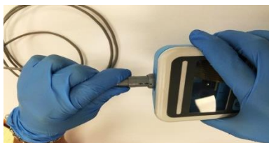
Figure 11: Plug antenna cable into AURA™ Monitor.
