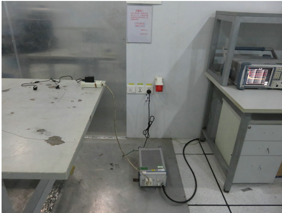
1 Photo of Conducted Emission Test
