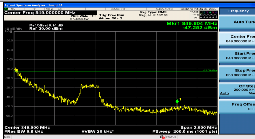
(Channel Bandwidth: 1.4 MHz)_HCH_16QAM_1RB#3
