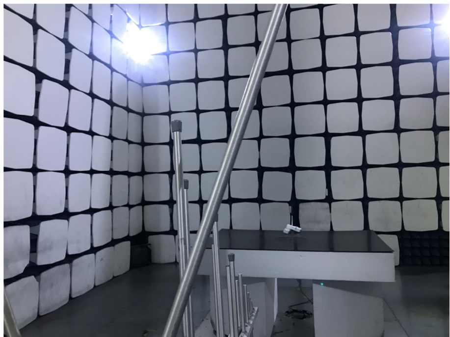
Radiation Emission Test Setup (30MHz to 1GHz)
